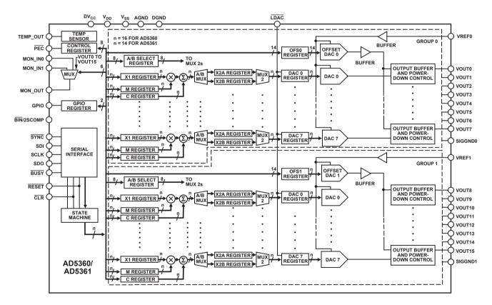
Figure 3. AD5360 Functional Block Diagram
