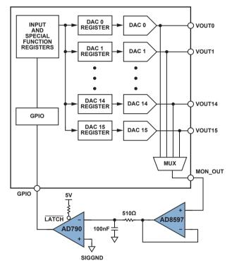
Figure 1. Circuit diagram.
